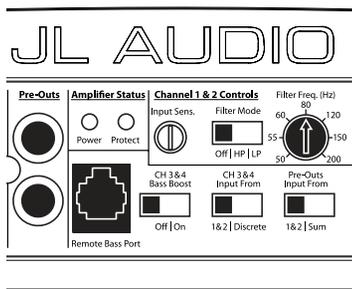
1) **“CH 3&4 Bass Boost”**: Found in the **“Channel 3 & 4 Controls”** section, this switch allows the user to activate a 6 dB boost centered at 48 Hz for channels 3 & 4. When the **“CH 3&4 Bass Boost”** is activated, the inputs to **“CH 3 (Left)”** and **“CH 4 (Right)”** are summed to create a mono signal. The **“Filter Mode”** switch in the **“Channel 3 & 4”** section must be in the **“LP”** position for the bass boost to be functional.
